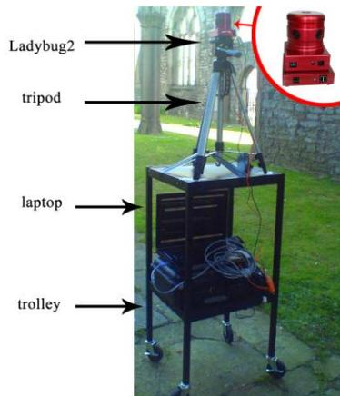
Figure 5. Ladybug2 – the spherical video camera inside the ruin of Charles Church. The application of a trolley for mobile camera approach.
