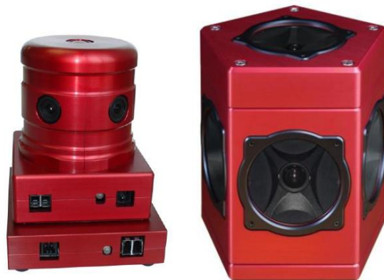
Figure 1 Ladybug 2 and Ladybug 3 – spherical video cameras produced by Point Grey Research
