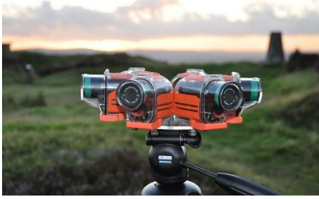
Figure 16 Six HD cameras create a 360° rig which generates cylindrical video panoramas.
