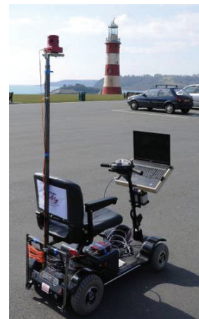
Figure 6: A motorised scooter provided by More Than Mobility from Plymouth was adjusted to be used with Ladybug2 camera
