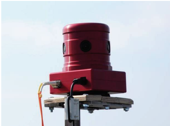
Figure 4: Ladybug2 – Spherical Digital Video Camera from Point Grey Research
