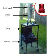
Figure 5. Ladybug2 – the spherical video camera inside the ruin of Charles Church. The application of a trolley for mobile camera approach.
