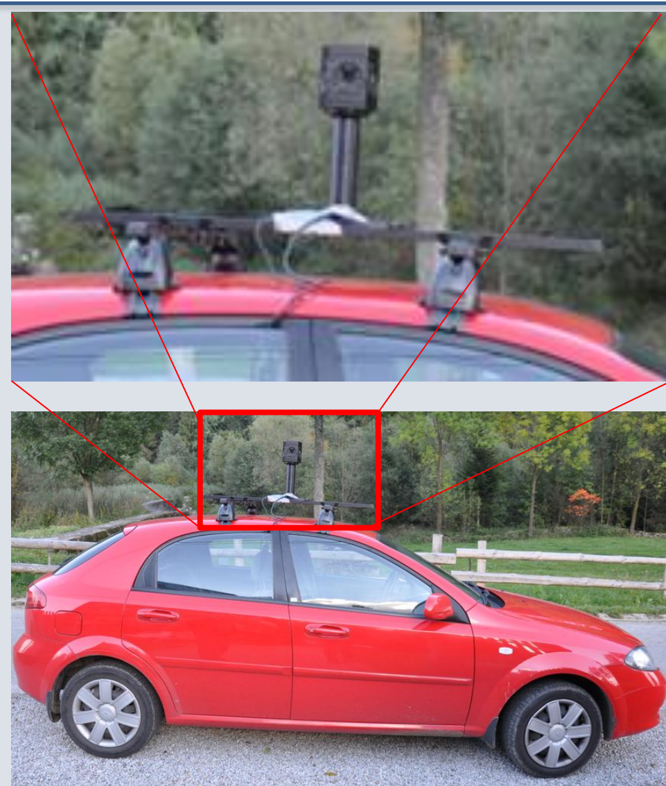
Immersive video camera mounted on a car
