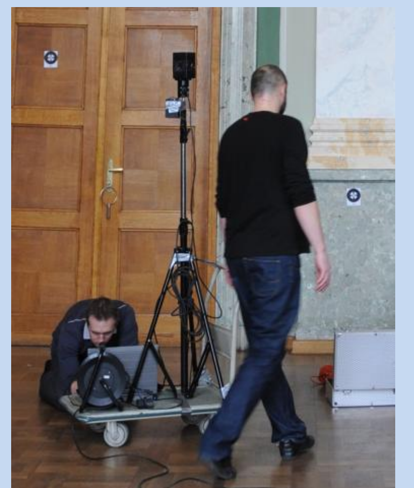
Immersive video camera mounted on a trolley
