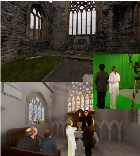
Figure 6. Lucid Viewer can display a movement of a person in a panoramic environment, that was recorded using chroma keying technique.
